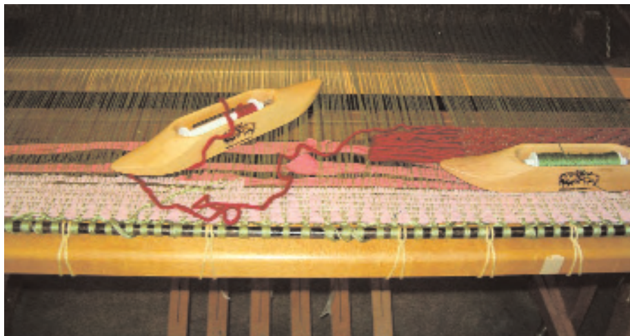
▲ Flying shuttle The shift from handloom to power loom for weaving made the manufacture of cloth much faster.
